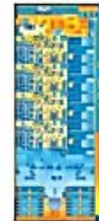
3rd generation Intel ® Core ™ processor Initial clock speed: 2.9GHz Transistors: 1.4 billion Manufacturing technology: 22nm
