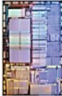
Intel 486 ® processor Initial clock speed: 25MHz Transistors: 1.2 million Manufacturing technology: 1 micron
